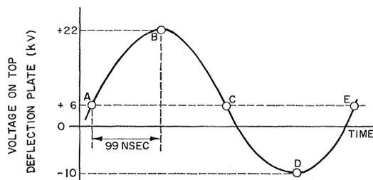
FIG. 2. Illustrating the operation of the rf beam gate. The beam pulses are shown as circles labeled A through E. Only pulse D is transmitted.
