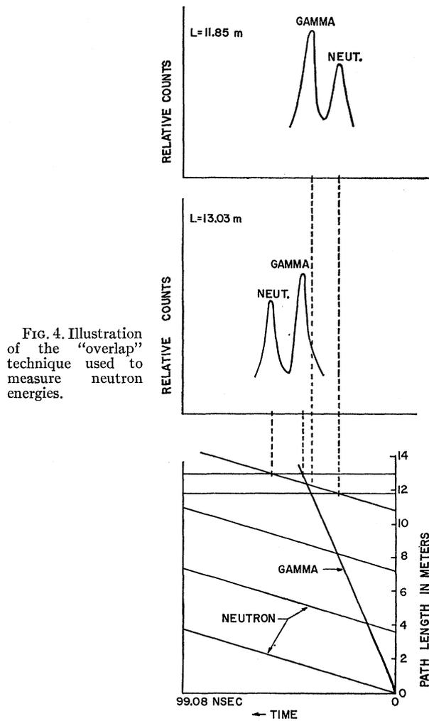
FIG. 4. Illustration of the "overlap" technique used to measure neutron energies.
